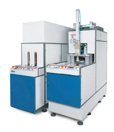
Acquired perfect reputation and well service-tested series of semi-automatic blow molding machines consists of UPF-5 and UPF-10 models. This universal series has been renewed with a semi-automatic blow molding machine UPF-30, designed for PET bottles 10-40 l production.
